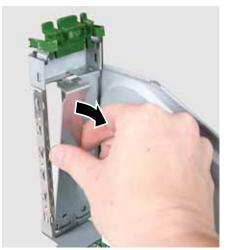
5 Slide a PCI card into the PCI slot, or slide a graphics card into the graphics card slot. You can slightly seesaw the card end-to-end to help insert the card, but do not bend the card sideways.
